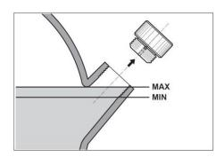
> Ensure the oil level in the Air End is to the level as shown.
