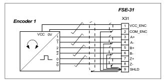
**Note**: This diagram is applicable to all revisions of FSE-31. However, VCC is 15 V DC for revision F and later, and 24 V DC for the module revisions A to E. You can see the revision of the module on the type designation label. Refer to *Type designation label* on page 18.
