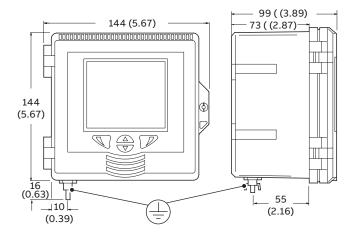
Figure 7 Transmitter dimensions
