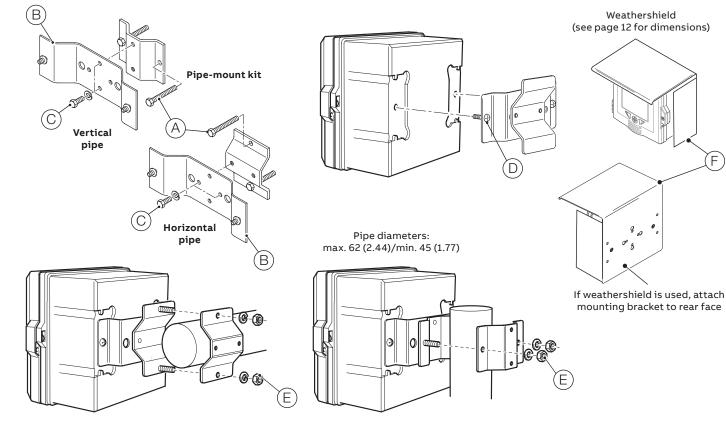
Figure 12 Pipe mounting the transmitter
