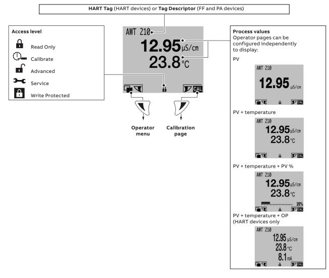
Figure 15 Example Operator pages – normal conditions
