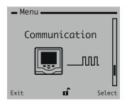
Communication level menus are enabled only if an optional communications module is fitted.
