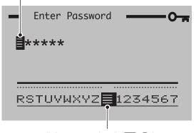
Cursor – scroll characters using the  $\bigcirc$   $\triangle$  keys; press  $\bigtriangledown$  (Next) to accept character; press  $\checkmark$  (OK) to accept password while last character is highlighted
