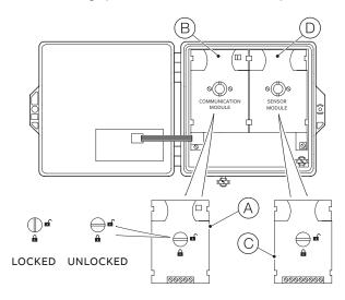
Figure 8 Fitting communication modules
