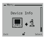
Displays read-only factory-set details for the transmitter software and connected sensor(s).
