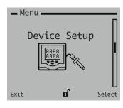
Used to setup security parameters, set PDM compatibility (for HART-enable transmitters) and to reset default (factory-set) parameters.
