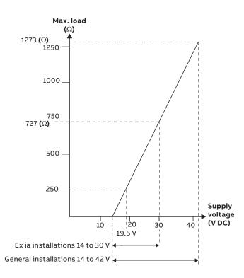
With 250  $\Omega$  resistor for HART communication min. supply voltage = 19.5 V DC
