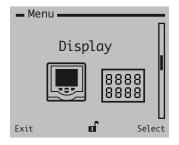
Used to setup **Operator pages (1, 2)**, select the display language and set the display contrast.
