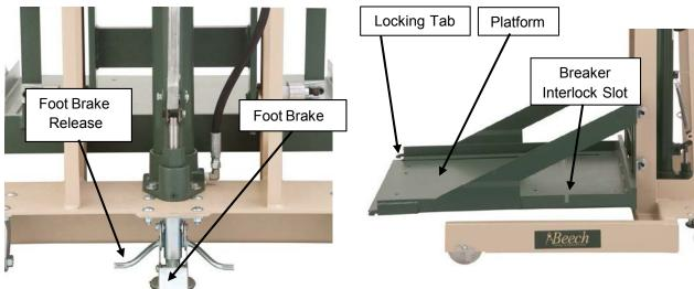
Figure 16: Lift truck foot brake
