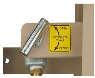
Figure 22: Lift truck control valve
