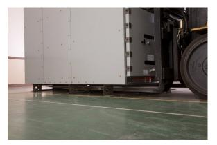
Figure 4: Complete fork penetration of all 3 shipping channels
