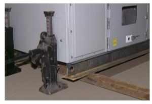
Figure 6: Placement of jacks at the corners with rollers under the shipping bases.
