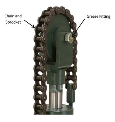
Figure 32: Lift Truck chain and sprocket
