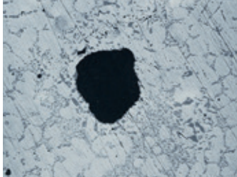
Hydrogen-induced porosity in castings
