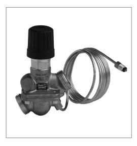
AHPBM-F is a self-acting differential pressure controller with flow limitation primarily for use in direct-connected district heating systems <u>with mixing loop only</u>. The controller closes on rising differential pressure or when set max. flow is exceeded.
