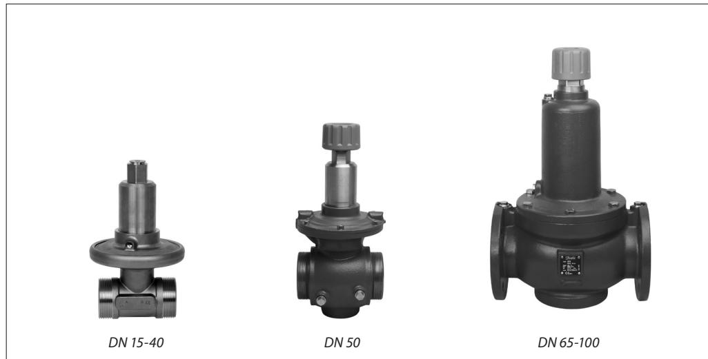
AHP is a self-acting differential pressure controller primarily for use in district heating systems or in secondary district heating systems as well. The controller closes on rising differential pressure.
