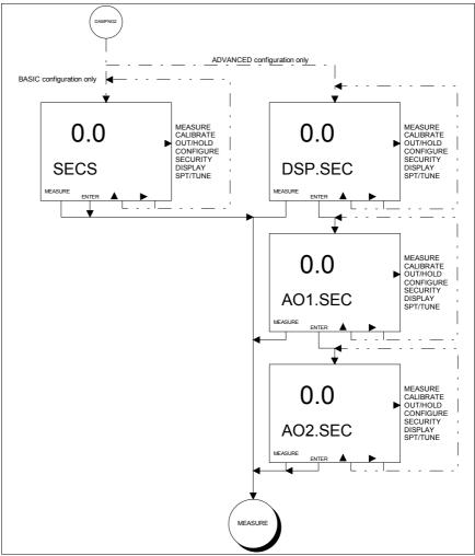
Figure 7-5. Screen Flow Diagram For Output/Hold Damping State
