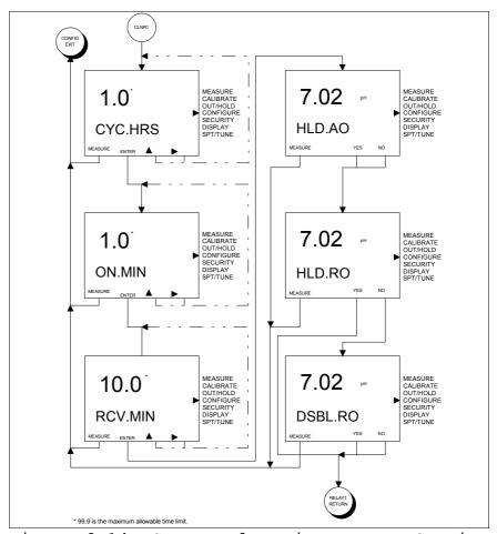
Figure 8-14. Screen Flow Diagram For Setting Damping State (Basic/Advanced) Relay Output Configure State of
