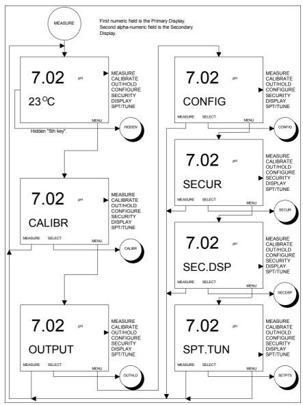
Figure 5-1. Screen Flow Diagram For Mode of Operation.
