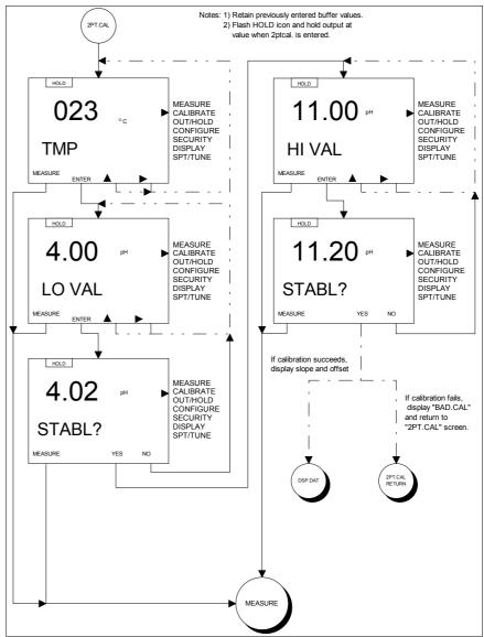
Figure 6-3. Screen Flow Diagram For Two-Point Process Calibration.
