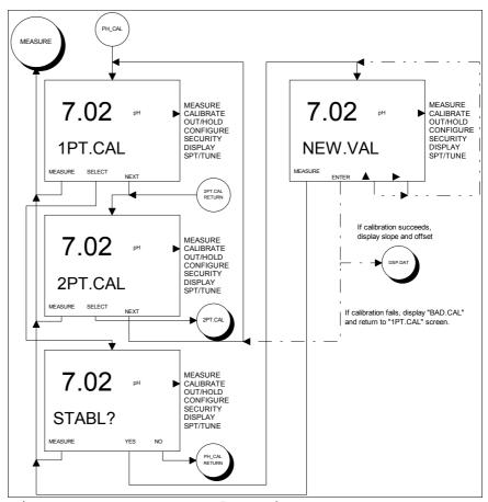
Figure 6-2. Screen Flow Diagram For Process Sensor Calibrate State of Operation.
