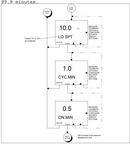
Figure 8-13. Screen Flow Diagram For Setting the Cycle Timer Relay Output Configure State Set Operation Timer parameters of a Relay Output using Figure 8-13 as reference and the following procedure:
