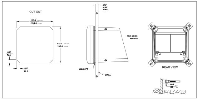
Figure 3-5. Panel Mount Installation Diagram
