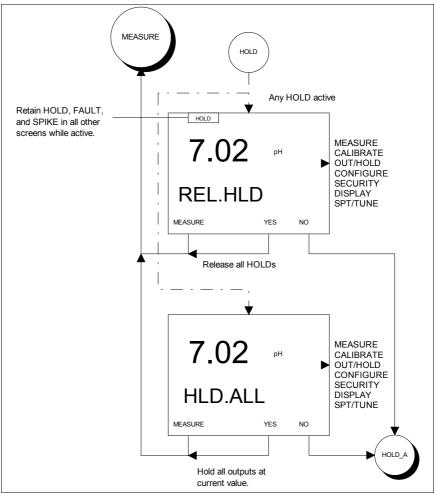
Figure 7-2. Screen Flow Diagrams For Hold State of Operation 7-1, an active Hold condition can be completely removed or manually altered. If a Hold condition is not active, the option to Hold All (i.e., HLD.ALL) In the latter case, confirmation is given. of this action using the YES Key causes the TB84PH Advantage Series analyzer to hold all analog and relay outputs at the levels and states captured when confirmation is made.
