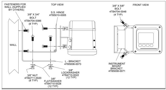
Figure 3-3. Hinge Mount Installation Diagram Wall Mounting
