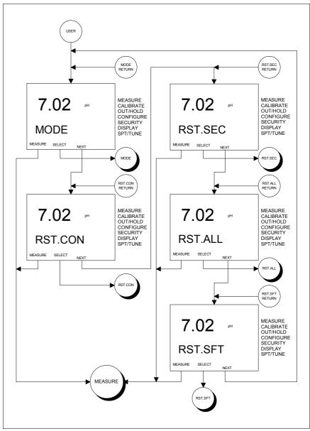
Figure 12-1. Screen Flow Diagram For User States of Operation.
