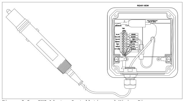
Figure 3-8. BNC Adapter Installation and Wiring Diagram
