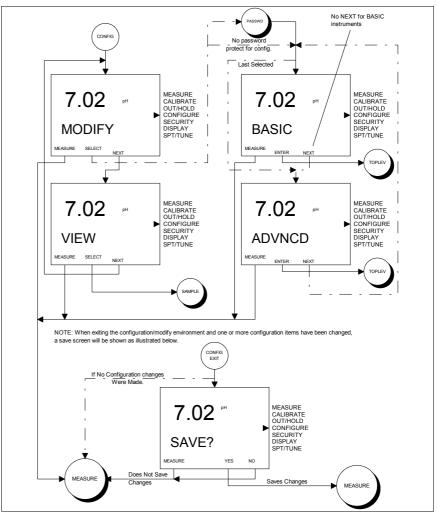
Figure 8-1. Screen Flow Diagram For Modify/View and Basic/Advanced Configure AsatsesnofinOperguien8-1, the TB84PH Advantage Series analyzer queries if the user would like to Modify the configuration. Pressing the YES Smart Key moves the user into the Modify Configure State, pressing the NO Smart Key moves the user to the View configuration query, and pressing the Exit To MEASURE Smart Key escapes to the Measure Mode.
