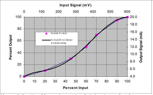
Figure 8-6. Non-linear Output Break Point Determination.
