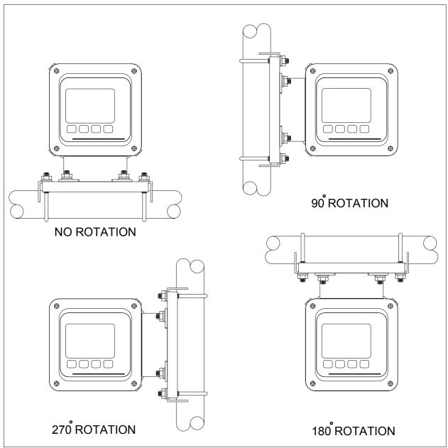
Figure 3-9. Mounting Rotation (Pipe Mount Shown)
