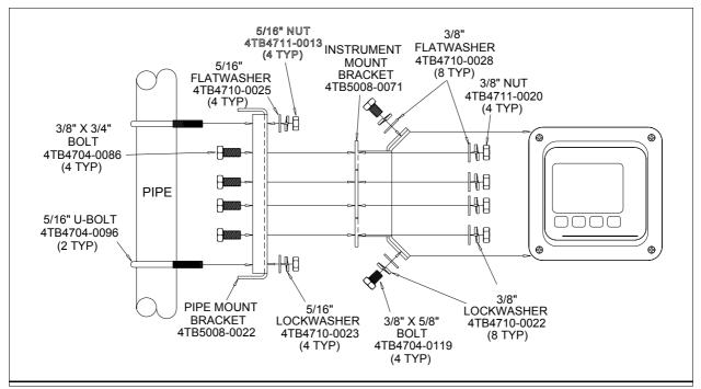
Figure 3-2. Pipe Mount Installation Diagram Hinge Mounting
