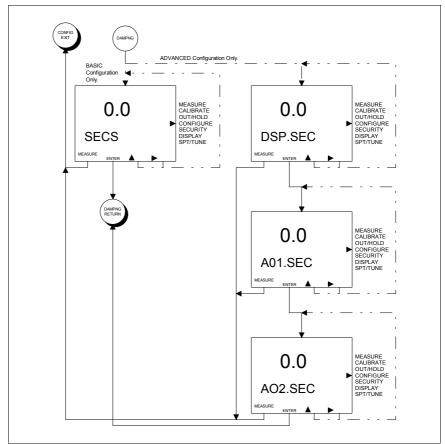
Figure 8-15. Screen Flow Diagram For Damping
