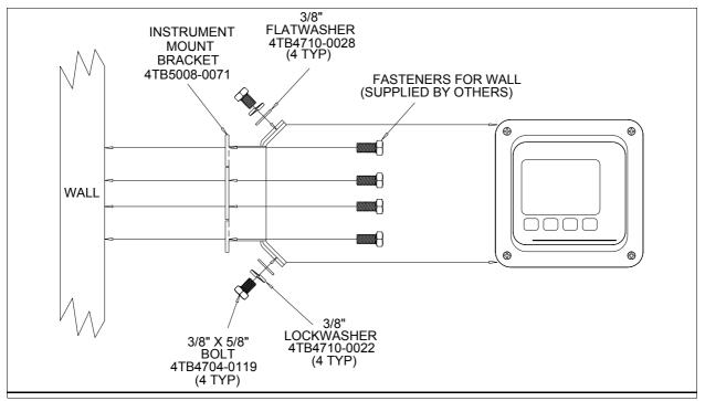
Figure 3 4. Wall Mount Installation Diagram Panel Mounting
