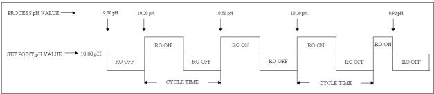
Figure 2.2. Cycle Timer High Set Point Example.
