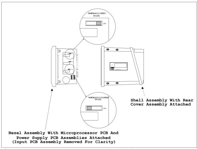
Figure 3-6. Normal State Relay Jumper Location.
