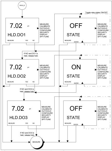
Figure 7-4. Screen Flow Diagram For Setting SpeciHoldReddy Outputs, StHtDsALL) outputs by pressing the YES Key, or hold specific outputs using the NO Key. Press the Exit To MEASURE Key to escape to the Measure Mode.
