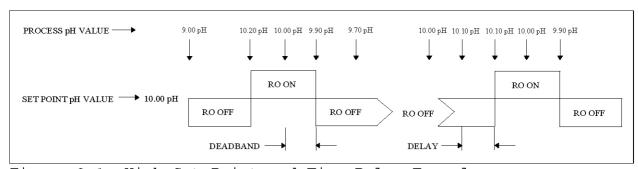
Figure 2-1. High Set Point and Time Delay Example. High or Low Cycle Timer
