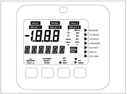
Figure 4-1. Fully Energized Display And Supporting Information. The top set of icons informs the user of an abnormal operating condition such as a output HOLD condition, FAULT condition, diagnostic SPIKE output, or RELAY activation. These icons are only energized when such a condition is detected and are active in all modes of operation.
