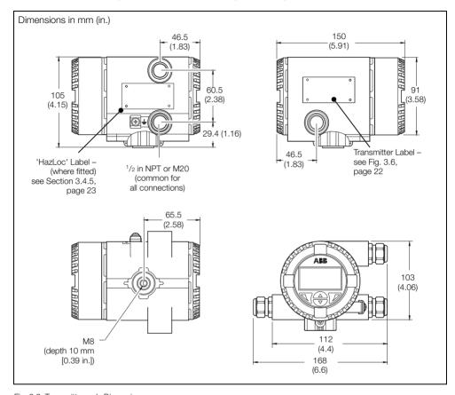
Fig. 3.3 Transmitter-only Dimensions
