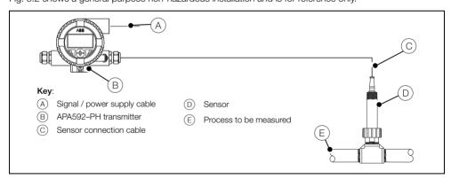
Fig. 3.2 Installation in Non-Hazardous Area
