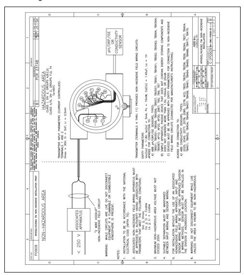
Fig. B.2 Installation Drawing P0909
