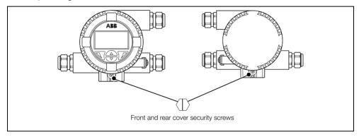
Fig. 3.1 Transmitter Cover Security Screws
