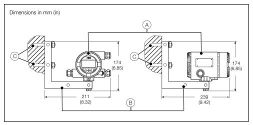
Fig. 3.4 Wall Installation
