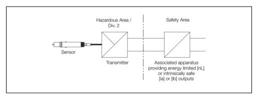
Fig. 4.13 Non-Incendive (using non-incendive field wiring) - FM and CSA
