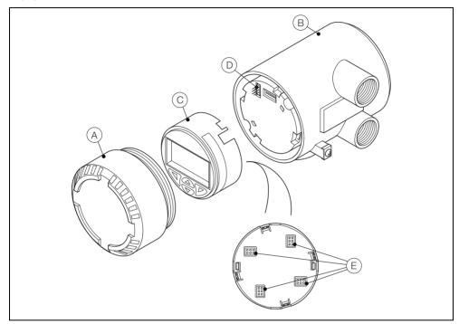
Fig. 3.10 LCD Display Alignment
