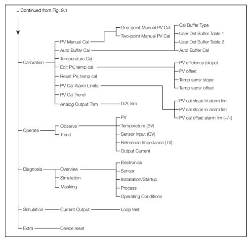
Fig. 9.2 HART Configuration Parameters (continued)
