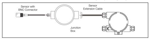
Fig. 4.5 Sensor with Junction Box and Extension Cable
