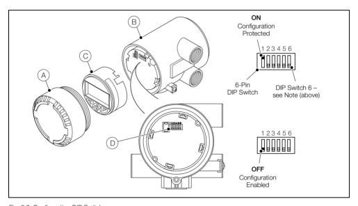
Fig. 6.2 Configuration DIP Switch
