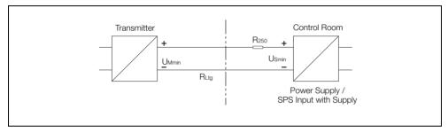
Fig. 4.8 Standard Application with HART Functionality
