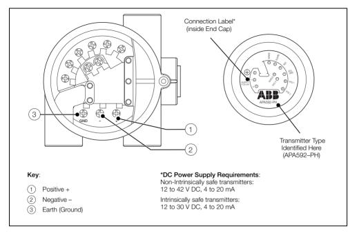
Fig. 4.2 Power Supply Connections at Transmitter Terminals
