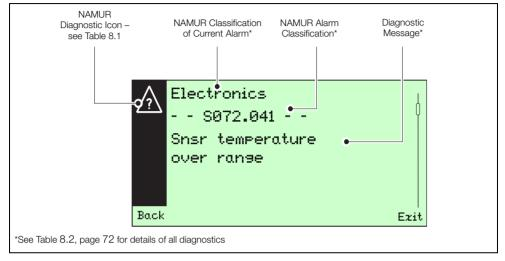
Fig. 8.1 Example of Diagnostic Alert
