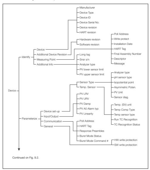
Fig. 9.1 HART Configuration Parameters
