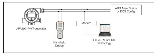
Fig. 6.1 Configuration Options - Schematic
