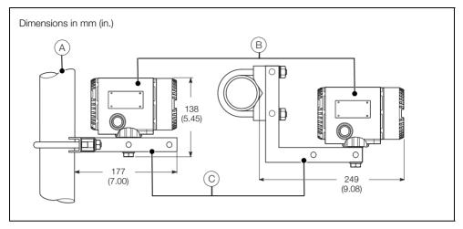
Fig. 3.5 Pipe Installation
