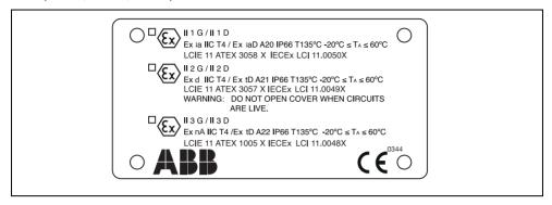
Fig. 3.7 Example of ATEX (Zone 0, Zone 1, Zone 2) 'HazLoc' Label
