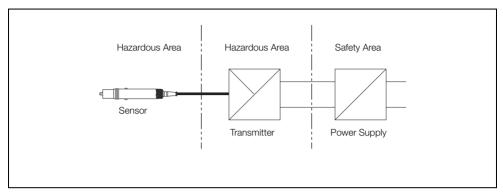
Fig. 4.12 Type n (Non-sparking) - ATEX/IECEx
