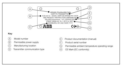
Fig. 3.6 Example of Transmitter Label (APA592-PH Version Shown)
