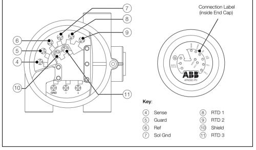
Fig. 4.3 APA592-PH Sensor Connections at Transmitter Terminals
