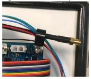
2. Attach the right angle SMA fitting of the cable to the board ANT-1, connector (J42).
