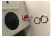
14. Secure the surge protector to the enclosure with the provided split washer and hex nut.
