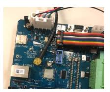
3. Attach the plug-to-jack adapter 4. Attach the surge protector to the straight SMA fitting of the cable.
