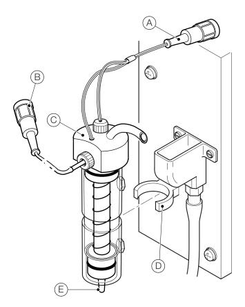
Figure 1 Hydrazine cell removal
