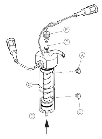
Figure 2 Hydrazine cell dismantling
