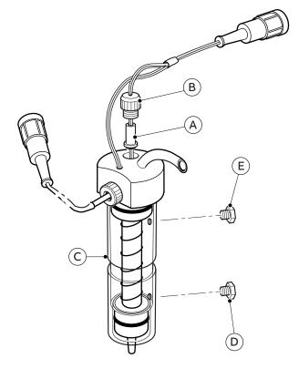
Figure 3 Hydrazine cell reassembly
