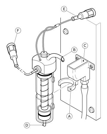
Figure 4 Hydrazine cell refitting
