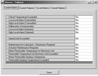
Figure 27: Screenshot of the detailed "Alarms / Failures" menu
