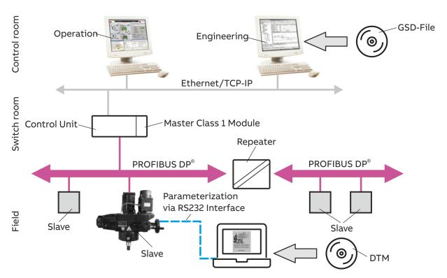
Figure 19: Arrangement of Contrac components for communication via PROFIBUS DP®
