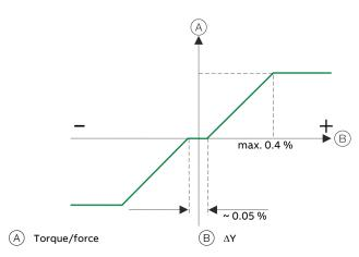
Figure 4: Torque / force depending on position deviation
