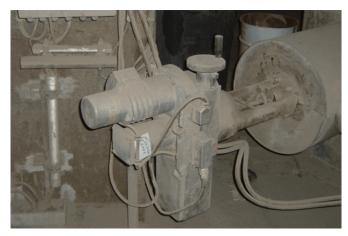
Figure 12: Horizontally mounted linear actuator
