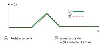
Figure 5: Schematic representation of a Contrac step response
