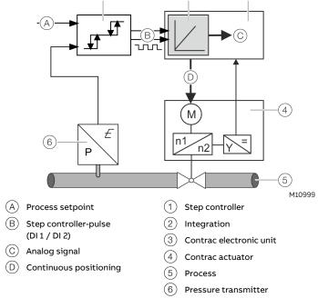
Figure 24: Integration of step commands into "Downstream from step controller" operating mode
