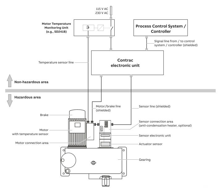
Figure 32: Allocation of the Contrac components when using in potentially explosive atmospheres (example)
