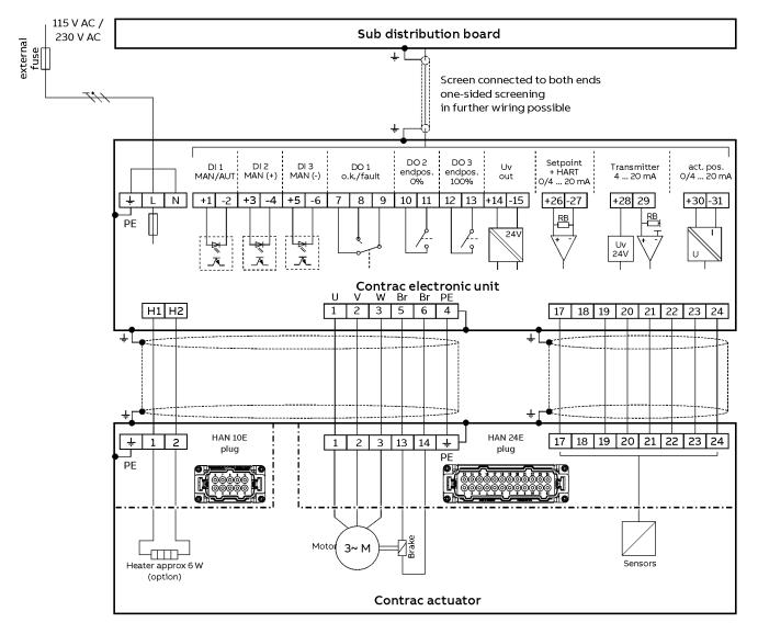
Figure 17: Wiring diagram (example based on field mounting of EBN853 / EBN861)
