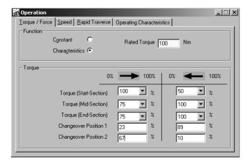
Figure 25: Screenshot of the menu for setting torque
