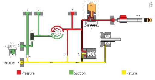
Before the burner starts the oil is heated in the oil preheater and in the nozzle line. This causes the oil to expand. The safety shut-off valve in the preheater prevents the oil from dripping out of the nozzle because the check valve B in the solenoid valve opens and thus makes a connection to the return or suction side of the pump. The preheater valve opens at a pressure  $\geq$  6 bar. The check valve B in the solenoid valve Opens at a pressure of max. 2 bar.
