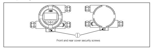
Fig. 3.1 Transmitter Cover Security Screws
