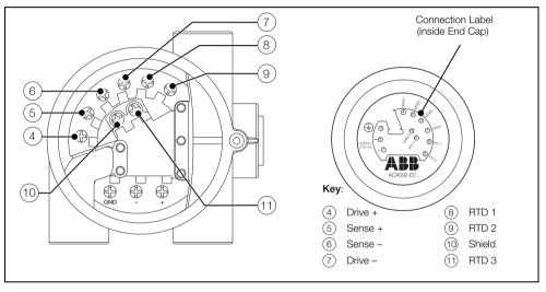
Fig. 4.3 ACA592-EC Sensor Connections at Transmitter Terminals
