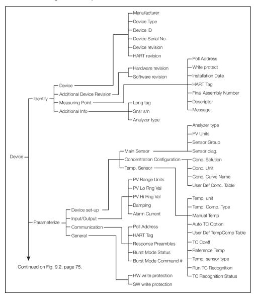
Fig. 9.1 ACA592 4-Electrode Conductivity Transmitter HART Configuration Parameters
