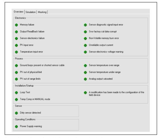
Fig. 8.2 ACA592 4-Electrode Conductivity Transmitter - Diagnosis Overview Screen
