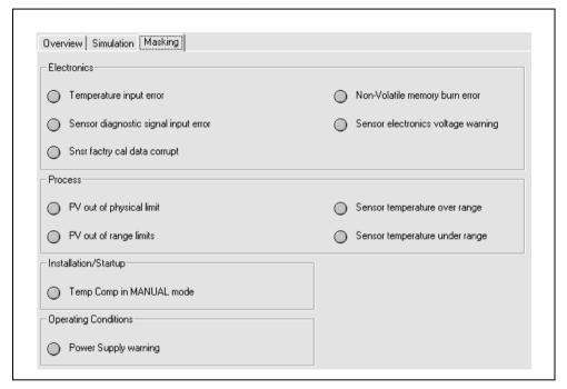
Fig. 8.3 ACA592 4-Electrode Conductivity Transmitter - Diagnosis Masking Screen
