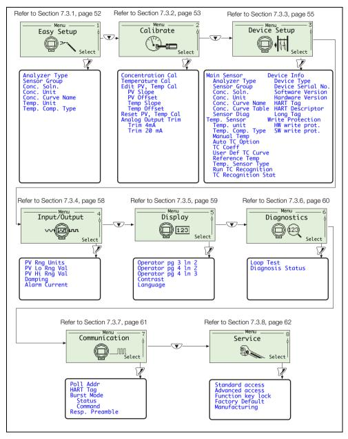
Fig. 7.4 ACA592 4-Electrode Conductivity Transmitter – Concentration Parameter Map
