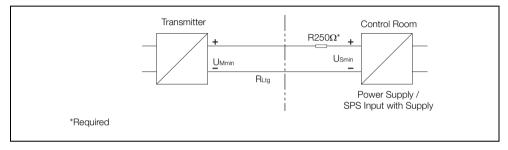
Fig. 4.7 Standard Application with HART Functionality
