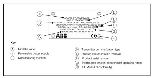
Fig. 3.6 Example of ACA592-EC Transmitter Label
