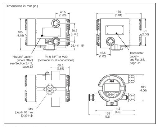
Fig. 3.3 Transmitter-only Dimensions
