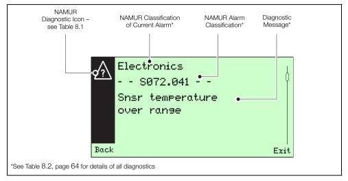
Fig. 8.1 Example of Diagnostic Alert
