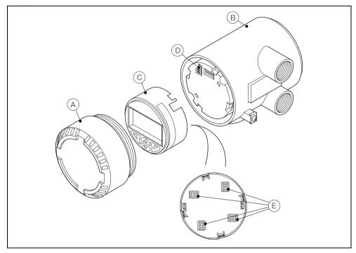
Fig. 3.10 LCD Display Alignment
