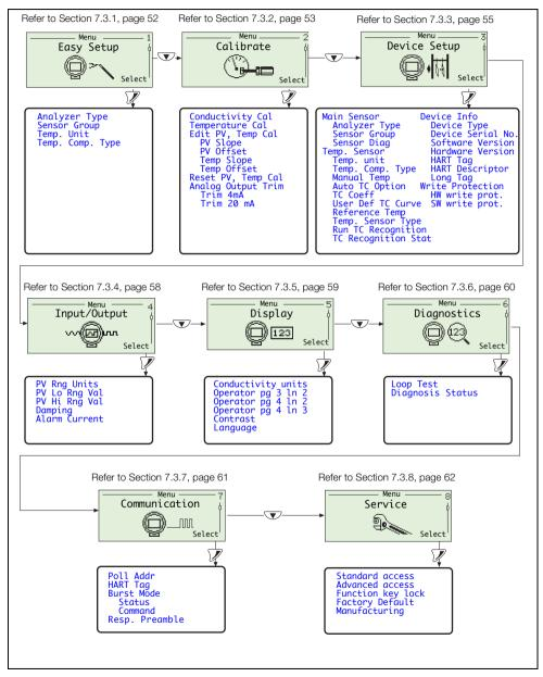
Fig. 7.3 ACA592 4-Electrode Conductivity Transmitter - Conductivity Parameter Map
