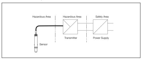
Fig. 4.11 Type n (Non-sparking) - ATEX/IECEX
