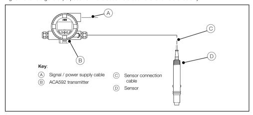
Fig. 3.2 Installation in Non-Hazardous Area
