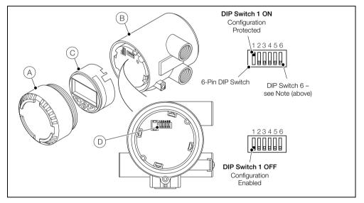
Fig. 6.2 Configuration DIP Switch
