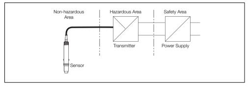
Fig. 4.13 Non-Incendive (using Div. 2 field wiring) - FM and CSA
