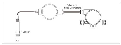
Fig. 4.5 Sensor with Junction Box and Extension Cable
