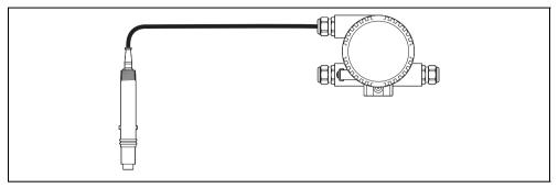
Fig. 4.4 Sensor with Integral Cable
