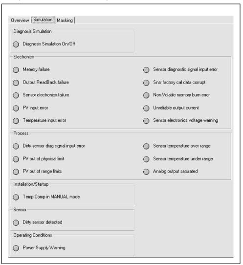
Fig. 8.4 ACA592 4-Electrode Conductivity Transmitter - Diagnosis Simulation Screen
