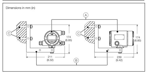
Fig. 3.4 Wall Installation
