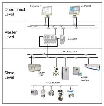
Fig. 2.1 Typical PROFIBUS Network
