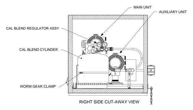
Figure 2–33 Calibration Bottle Location
