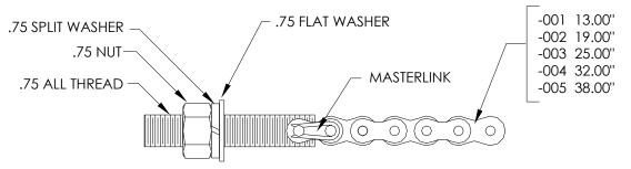
Figure 2–10 Adjustment Assembly
