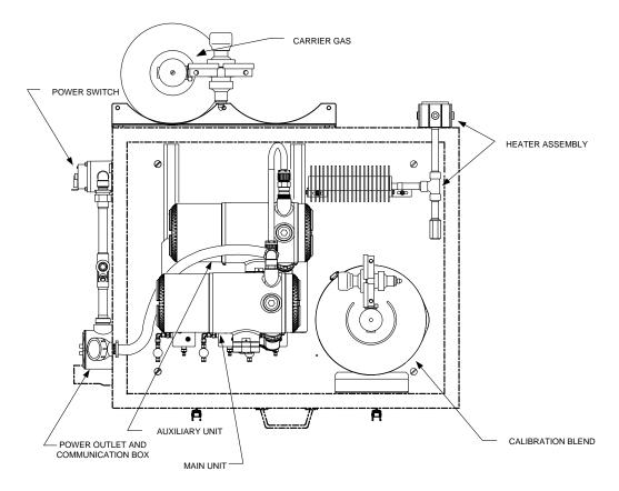
Figure 2–3 Typical Environmental Enclosure with Electric Heater
