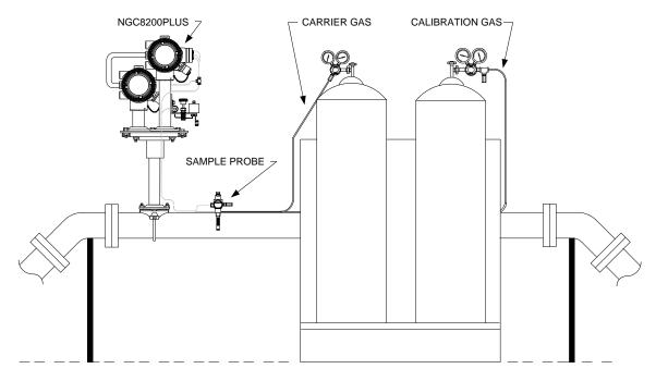
Figure 2–1 Basic Meter Run Installation
