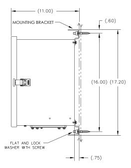
Figure 2–48 6200 Enclosure Wall Mounted Installation
