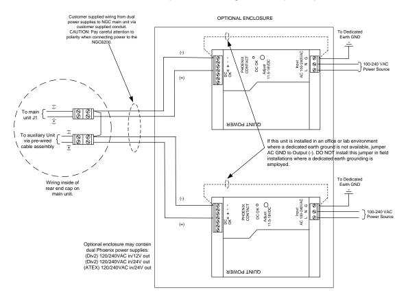
Figure 2–51 Dual Phoenix Power Supply AC and DC Wiring
