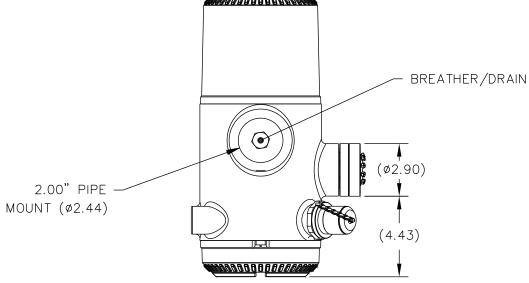
Figure 1–7 NGC8200 Enclosure Underside
