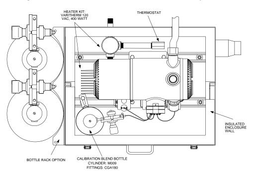
Figure 1–22 ENC82S Environmental Enclosure with Electric Heater
