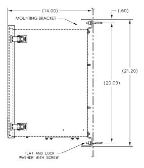
Figure 2–49 6700 Enclosure Wall Mounted Installation
