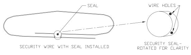
Figure 1–29 Security Wire with Seal
