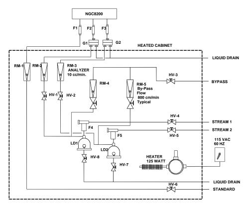
Figure 1–18 Typical Sample Installation Diagram
