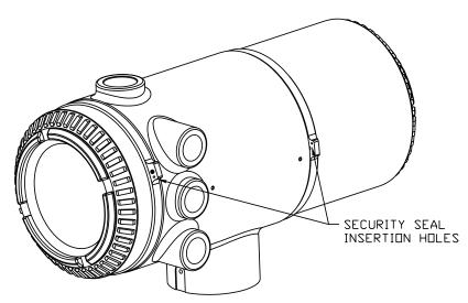
Figure 1–28 NGC End Cap Tabs for Security Seal
