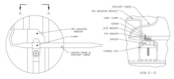
Figure 2–42 Temperature Probe Installation
