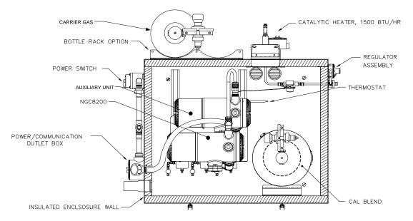
Figure 2–38 Catalytic Heater Option in ENC82
