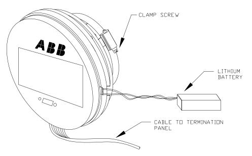
Figure 4–1 Digital Controller Complete assembly
