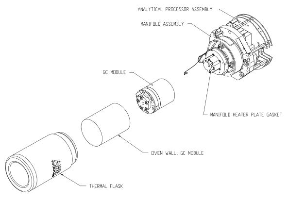
Figure 4–5 GC Module, Exploded View
