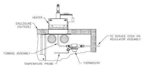
Figure 2–40 Thermostat Assembly Installed
