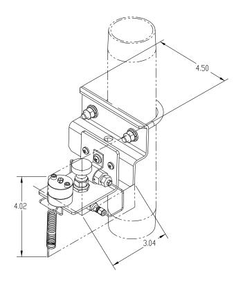
Figure 1–26 Single Stream Conditioning Module Dimensions
