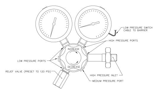
Figure 2–31 Carrier Gas Pressure Regulator with Relief Valve
