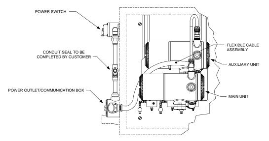
Figure 2–23 Assembled Power/Communication Assembly
