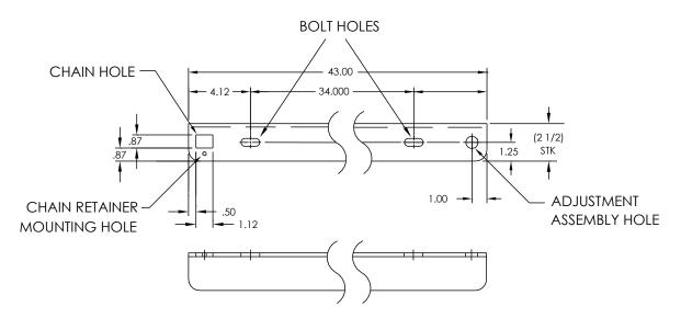
Figure 2–8 Mounting Brackets
