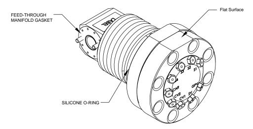
Figure 4–7 Feed-Through Assembly
