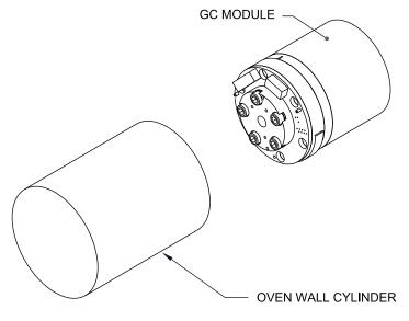
Figure 1–10 GC Module Assembly
