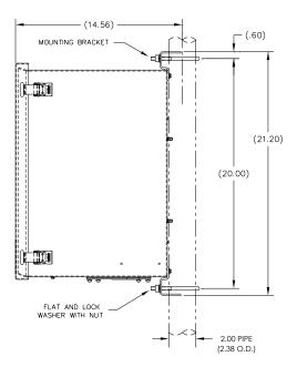
Figure 2–47 6700 Enclosure Pipe Mounting Installation
