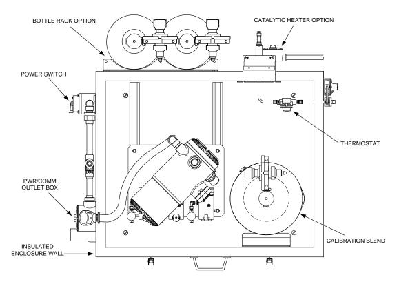
Figure 1–21 ENC82L Environmental Enclosure with Catalytic Heater
