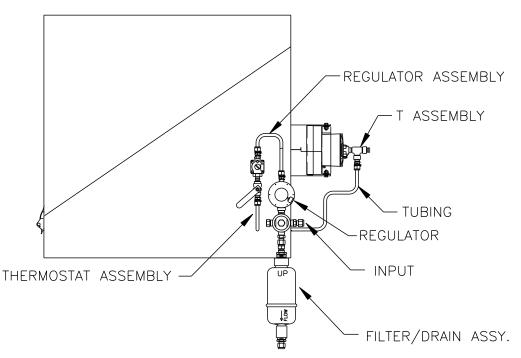
Figure 2–41 Regulator Assembly Installed
