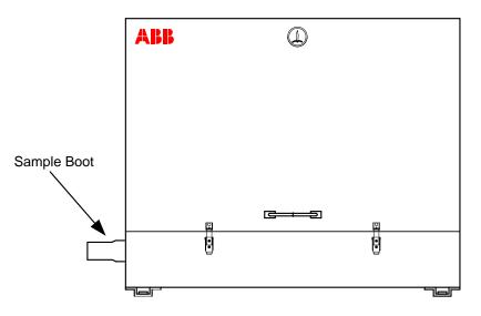
Figure 2–20 ENC82L–Environmental Enclosure Sample Boot
