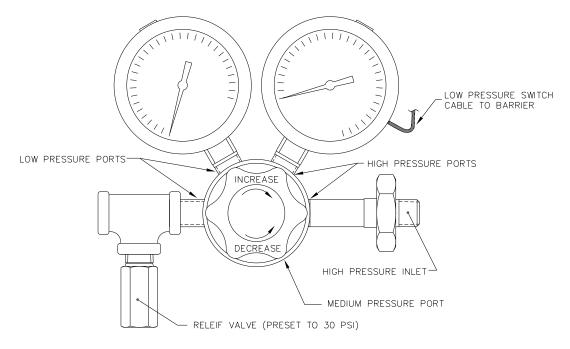
Figure 2–34 Calibration Gas Pressure Regulator with Relief Valve
