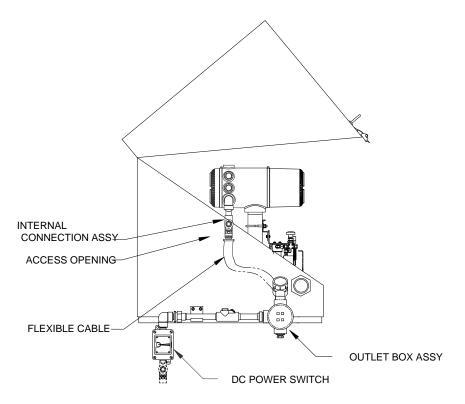
Figure 2–21 ENC82 External Power/Communication Assembly
