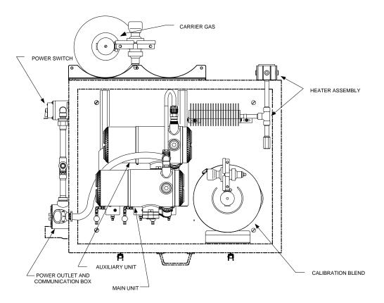
Figure 2–44 Electric Heater Installed in ENC82
