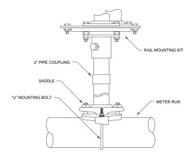
Figure 2–14 Typical Pipe Saddle Installation
