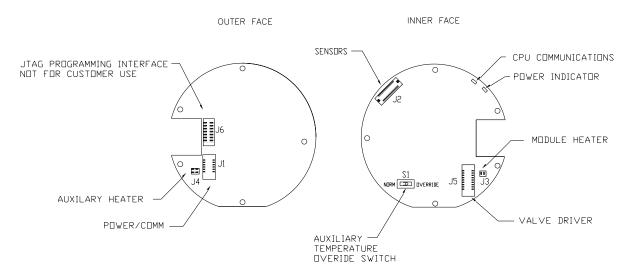
Figure 4–4 Analytical Processor Board
