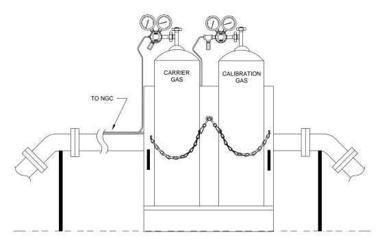
Figure 2–28 Carrier/Calibration Gas Bottle Rack Installation
