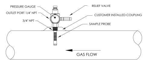
Figure 2–5 Sample Probe Insertion
