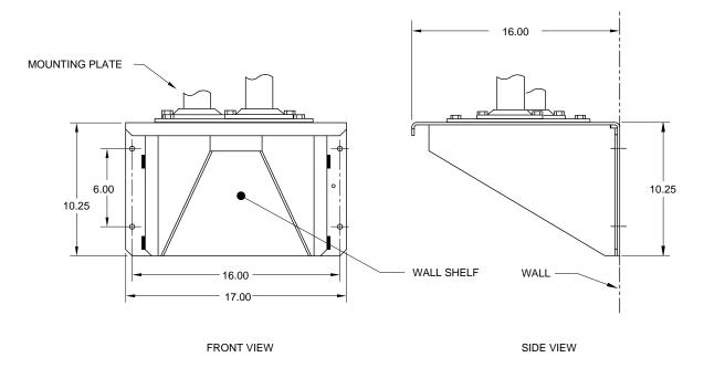
Figure 2–2 Typical Wall Shelf Mount Installation
