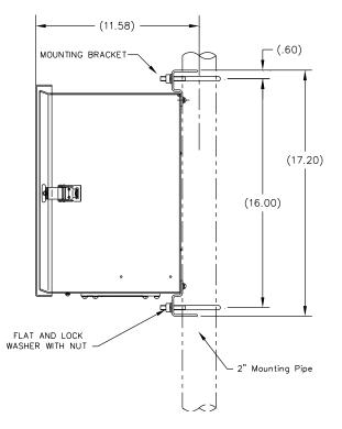
Figure 2–46 6200 Enclosure Pipe Mounting Installation
