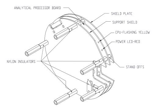
Figure 1–12 Analytical Processor Assembly
