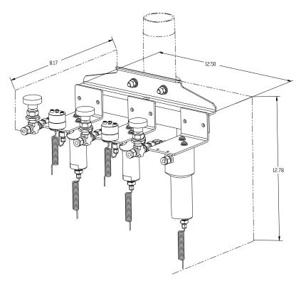
Figure 1–27 Multiple Stream Conditioning Module Dimensions
