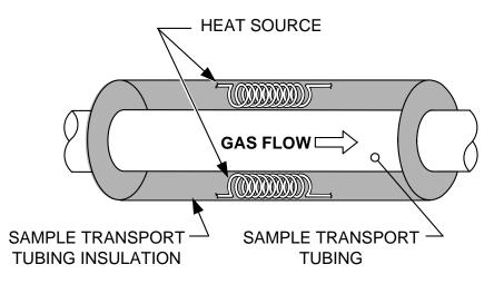
Figure 1–17 Heat Tracing Sample Line
