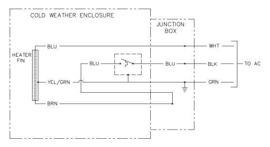
Figure 2–45 Electric Heater Option Wiring Instructions
