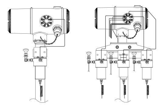
Figure 1–25 Single and Multiple Stream Sample Conditioning Assemblies
