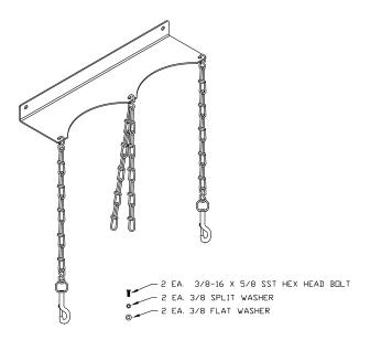
Figure 2–29 Dual Bottle Rack Assembly
