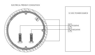
Figure 2–43 Electrical Pre-Heater Wiring Instructions
