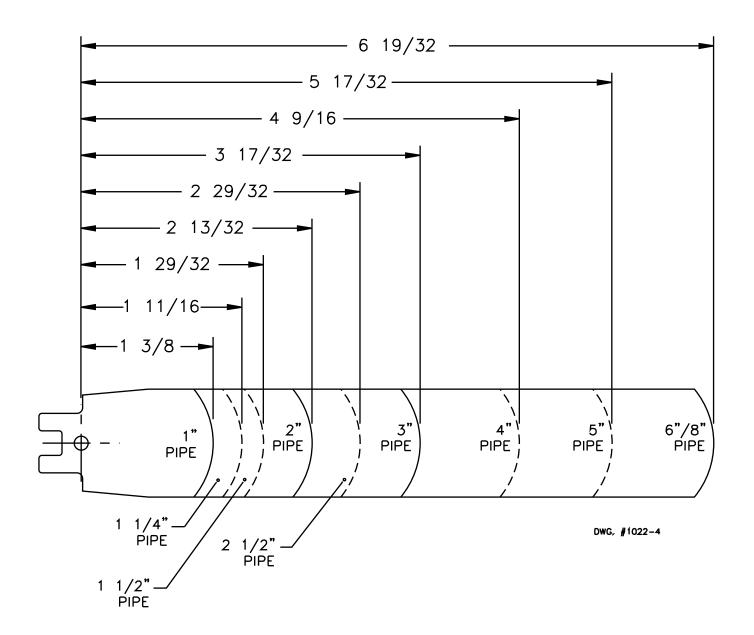
Flexible paddles smaller than the actual pipe size should be used for added support and higher sensitivity. See Fig. 2. The paddles must be properly attached and the screw that holds the paddle must be securely tightened.
