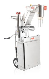
The LiMCA III uses the proven LiMCA measurement principle that is the industry benchmark for measuring non-metallic solid inclusions in molten aluminium.
