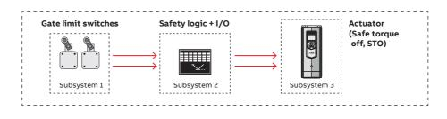
Figure 3-6: Structure of a safety function
