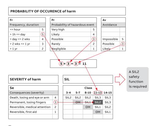
Figure 3-4: Example of SIL assignment table (based on EN/IEC 62061, tables A.1-A.4; A.6)
