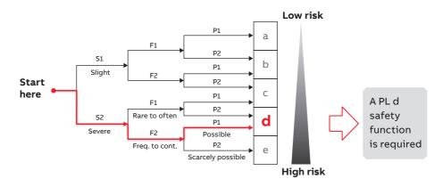
Figure 3-5: Example of PL risk graph (based on EN ISO 13849-1, figure A.1)
