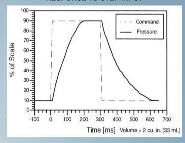
Fig. 2 Times for MM to fi II/exhaust a closed chamber. Step command signal is superimposed over pressure trace. Time is determined by difference between command signal and pressure achieved.
