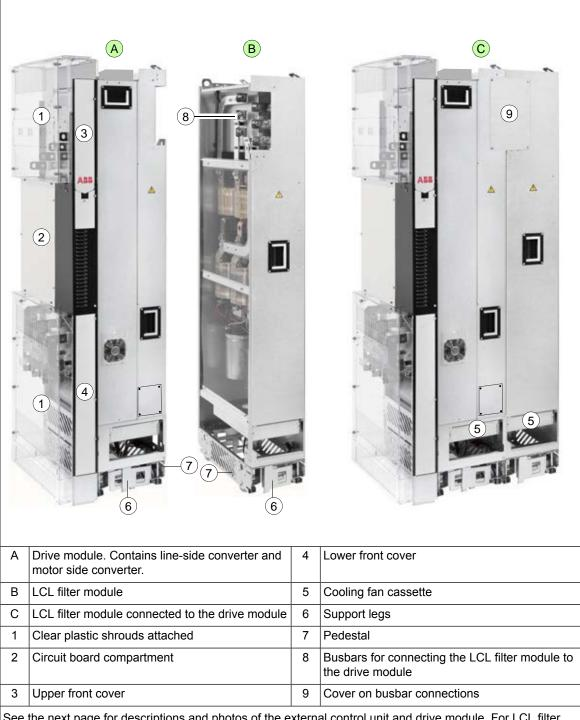
See the next page for descriptions and photos of the external control unit and drive module. For LCL filter module, see section *LCL filter module* (page 36).
