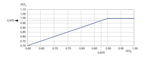
Example 1:  $P_n$  for ACS880-14-650A-3 is 355 kW. The input voltage (*U*) is 350 V. ->  $U/U_n$  = 350 V / 400 V = 0.875. ->  $P/P_n$  = 0.975 -> The derated power P = 0.975 × 355 kW = 346 kW.
