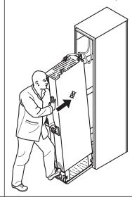
13 Unfasten the extraction/installation ramp and attach the LCL filter module to bottom plate.
