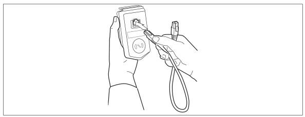
**Note:** When a PC is connected to the control panel, the control panel keypad is disabled. In this case, the control panel acts as a USB-RS485 adapter.
