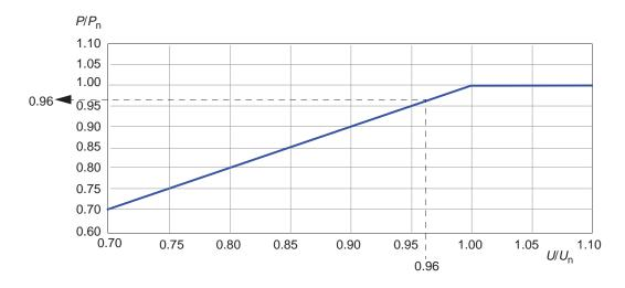
Example 1:  $P_{\rm n}$  for ACS880-14-430A-7 is 400 kW. The input voltage (*U*) is 660 V. ->  $U/U_{\rm n}$ = 660 V / 690 V = 0.96 ->  $P/P_{\rm n}$  = 0.96 -> The derated power P = 0.96 × 400 kW = 384 kW.
