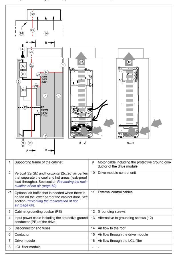
Note: The power cable shields can also be grounded to the drive module grounding terminals.
