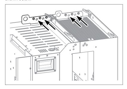
You can attach the modules to Rittal VX25 enclosure with the mounting brackets delivered with the drive, see *Step-by-step drawings for an installation example of standard drive configuration in Rittal VX25 800 mm wide enclosure (page 233)*.
