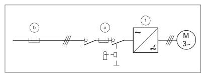
Size the fuses or the circuit breaker according to local regulations for the input cable protection. Select the fuses for the drive according to the instructions given in the technical data. The fuses for the drive protection will restrict drive damage and prevent damage to adjoining equipment in case of a short-circuit inside the drive.
