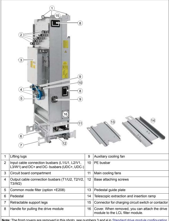
Note: The front covers are removed in this photo, see numbers 3 and 4 in Standard drive module configuration.
