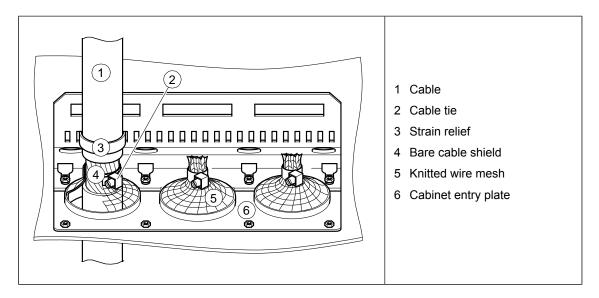
ABB recommends 360° high-frequency grounding of the control cable shields at their entries. The shields can be grounded by means of conductive shielding cushions pressed against the cable shield from both directions as shown below.
