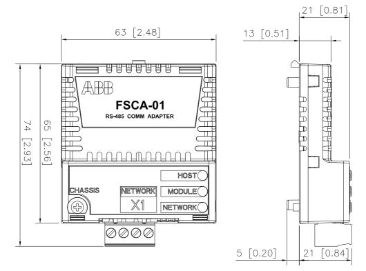
Mounting: Into the option slot on the drive
