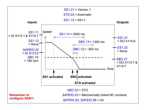
**Example 2:** The figure below shows an example of the SS1-r function with speed limit activated SBC, SBC before STO set-up:
