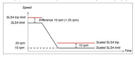
Example 2: The original SLS4 and SLS4 trip limits are: 1000 and 1100 rpm. The scaling value is 0%. The zero speed value is 20 rpm.
