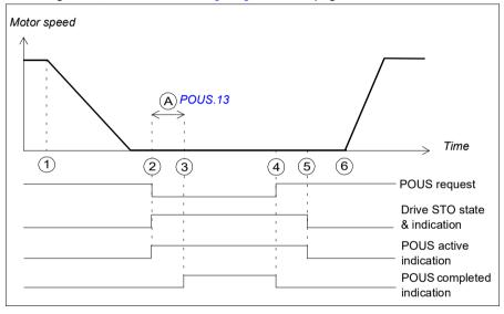
Α POUS delay for completion (parameter POUS.13): An additional security delay. The POUS completed indication (parameter POUS.22) goes on after this delay.
