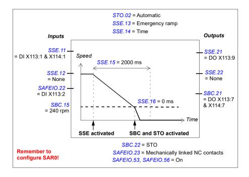
**Example 2:** The figure below shows an example of the SSE with emergency ramp function with speed limit activated SBC set-up with ramp monitoring:
