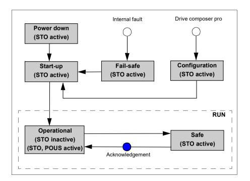
At power-up, the FSO goes into the Start-up mode: it performs start-up checks and. according to the configuration, enters the Operational state either automatically or after an acknowledgement request from the FSO I/O or from a safety PLC.
