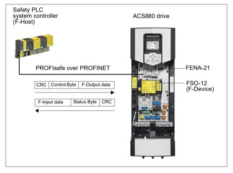
The FSO safety functions module and the FENA-21 Ethernet adapter module are installed on the ACS880 drive. The safety PLC is connected to the FENA module, which communicates with the FSO module. The safety PLC activates safety functions via the PROFIsafe communication bus. The user can also activate safety functions from an I/O device (for example, an emergency stop button) which is connected to the FSO module
