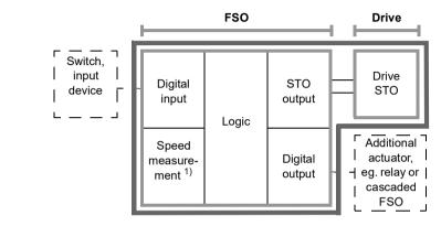
The safety data of the FSO and the drive is composed of the safety data of the subsystems used in the FSO and the safety data of the drive STO.
