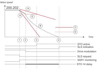
SLS request is activated (SLSx.11 SLS1 input A = DI X113:2 & X114:2). SLS ramp monitoring is activated (SAR1). Parameter 200.202 SAR speed scaling (=
