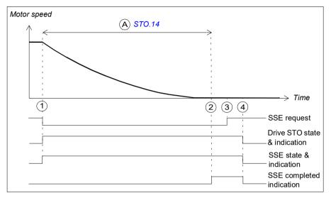
Α Time to zero speed (parameter STO.14): Time from the STO activation to the moment when the safety function is completed, the SSE completed indication (parameter SSE.22) goes on and the acknowledgment becomes allowed. You must set this to the estimated time in which the motor coasts to a stop from the maximum speed.
