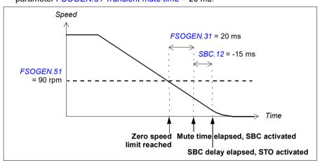
Note: If the SBC delay (parameter SBC.12 STO SBC delay) is positive or zero (0 ms), the SBC and STO functions are activated at the same time.
