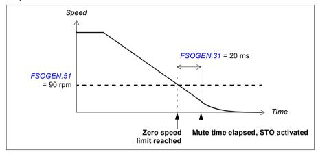
Example 2: Zero speed limit in reached in the SS1 function (and SSE with emergency ramp), a negative SBC delay (parameter SBC.12 STO SBC delay) is configured in the STO function:
