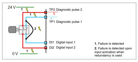
Note: If only one of the redundant inputs is activated upon a safety function request, the FSO module activates the safety function but it cannot be acknowledged before the failure has been repaired. To acknowledge the safety function, you must set both input channels down and up at the same time or, switch the power off and on.
