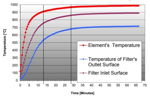
Figure 2: Filter Temperature During Preheating on the Crucible Heater
