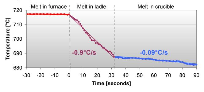
Figure 1: The most significant heat loss occurs when the metal is in the ladle (see PoDFA Eng Bulletin No. 1)
