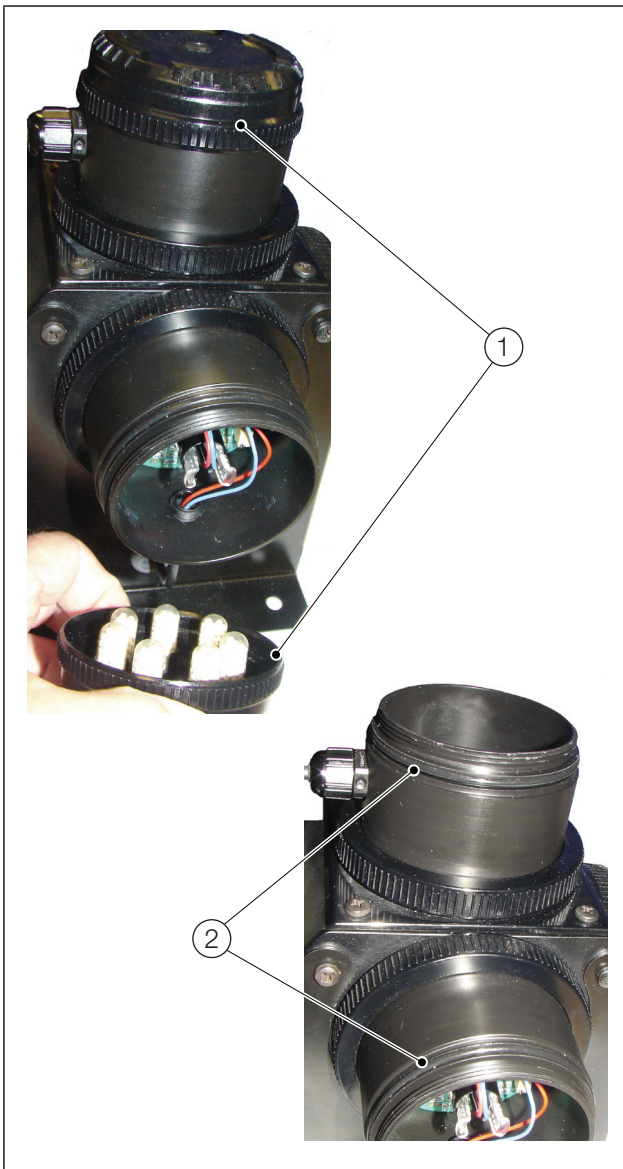
Fig. 3.1 End cap replacement
