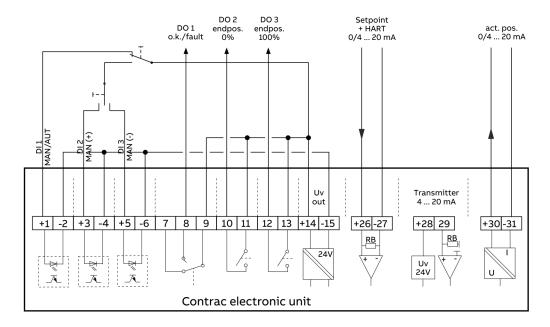
Figure 13: Connection example for operation following a continuous set point (standard configuration)
