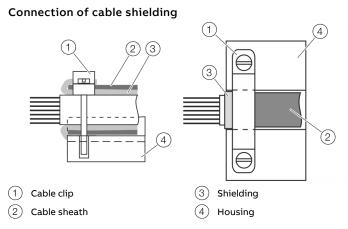
Figure 16: Cable shielding
