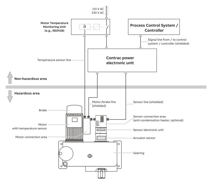
$\textbf{Figure 1:} \quad \textbf{Allocation of the Contrac components when using in potentially explosive atmospheres (example) } \\$
