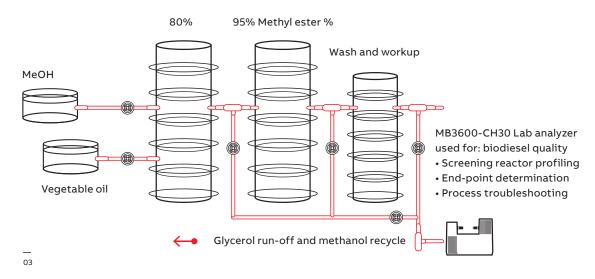
The MB3600-CH30 laboratory FT-NIR analyzer is designed and configured for routine biodiesel analysis and easy calibration modeling and method preparation. It includes all the hardware, software and accessories required for both biodiesel measurement and chemometrics method development.
