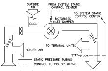
SUPPLY FAN CAPACITY CONTROL FOR VARIABLE AIR VOLUME SYSTEM
