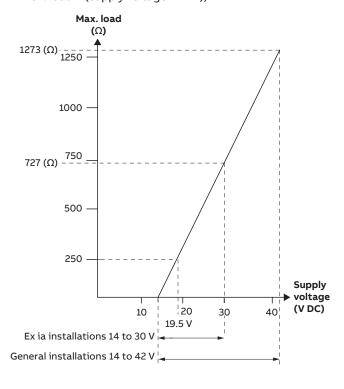
With 250  $\Omega$  resistor for HART communication min. supply voltage = 19.5 V DC
