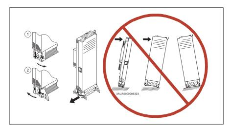
• To prevent the drive module from falling, attach its top lifting lugs with chains to the cabinet (1) before you push the module into the cabinet and pull it from the cabinet. Push the module into the cabinet and pull it from the cabinet carefully preferably with help from another person. Keep a constant pressure with one foot on the base of the module (2) to prevent the module from falling on its back.
