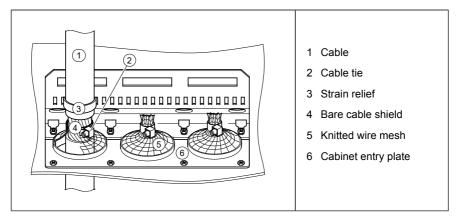
• ABB recommends 360° high-frequency grounding of the control cable shields at their entries. The shields can be grounded by means of conductive shielding cushions pressed against the cable shield from both directions as shown below.
