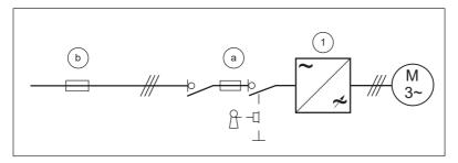
Size the fuses or the circuit breaker according to local regulations for the input cable protection. Select the fuses for the drive according to the instructions given in the technical data. The fuses for the drive protection will restrict drive damage and prevent damage to adjoining equipment in case of a short-circuit inside the drive.
