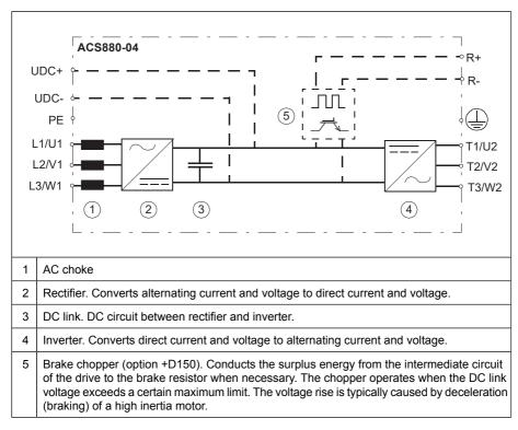
The main circuit of the drive module is shown below.
