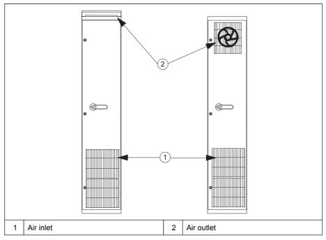
Arrange the cooling air flow through the components according to the technical data. See the specifications for:
