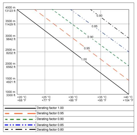
can be reduced by 1.5% for every 1 °C reduction in temperature. For a more accurate derating, use the DriveSize PC tool. A few altitude derating curves are shown below.
