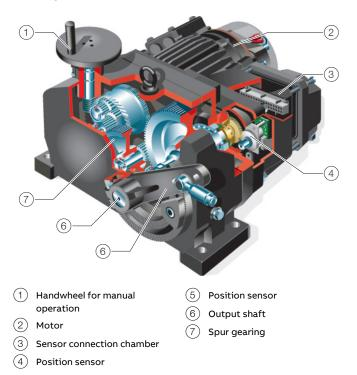
Figure 1: Cross-section of a rotary actuator (example)
