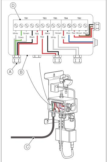
Fig. 6.7 Replacing the Modbus cable assembly
