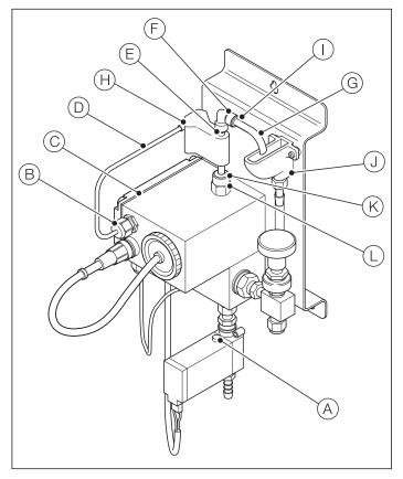
Fig. 6.4 Replacing the flowmeter assembly
