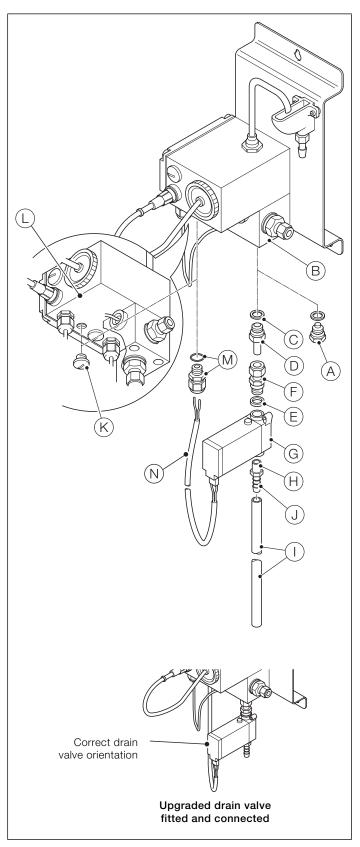
Fig. 7.2 Upgrading the drain valve assembly
