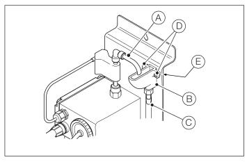
Fig. 6.3 Replacing the tundish assembly
