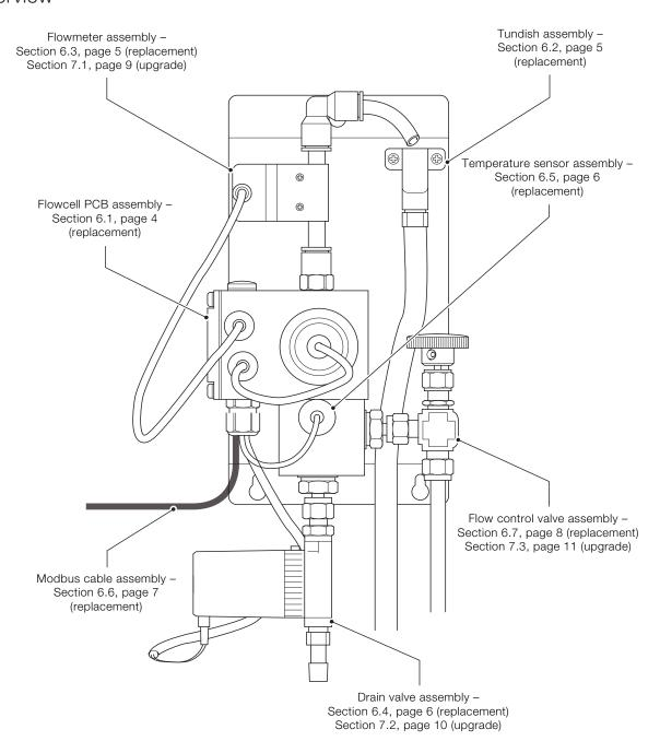
Fig. 5.1 ADS551 Wet section spares - item locations
