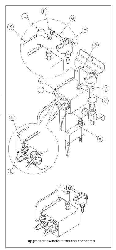
Fig. 7.1 Upgrading the flowmeter assembly
