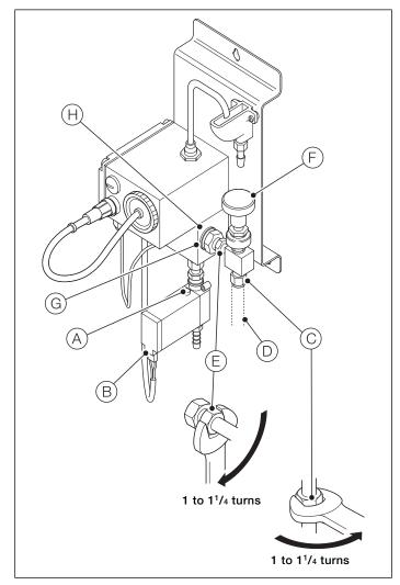
Fig. 6.8 Replacing the flow control valve assembly
