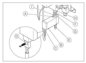
Fig. 6.5 Replacing the drain valve assembly and drain valve cable assembly
