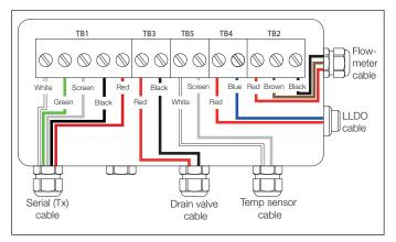
Fig. 6.2 Cable connections to transmitter - ADS551
