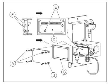
Fig. 6.1 Replacing the flowcell PCB housing gasket, PCB housing and PCB
