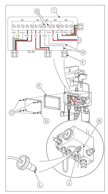
Fig. 6.6 Replacing the temperature sensor assembly
