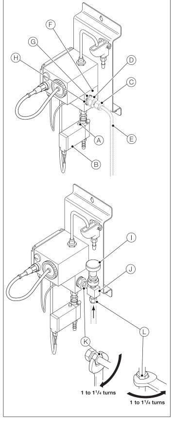
Fig. 7.3 Upgrading the flow control valve assembly
