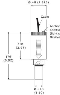
Anchor point for additional support (light chain or flexible cable)
