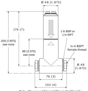
Note. Allow an additional 130 mm (5.125 in) for connectors and cartridge removal.
