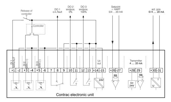
Figure 13: Connection example for operation downstream from a step controller
