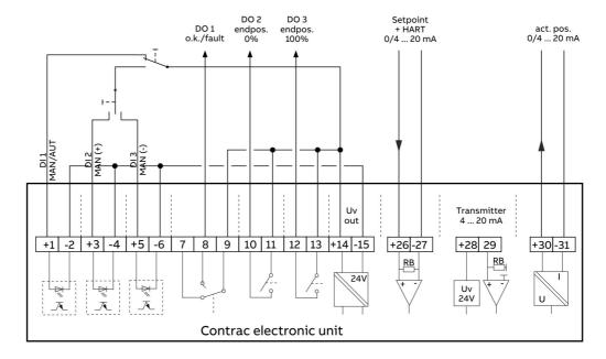
Figure 12: Connection example for operation following a continuous set point (standard configuration)
