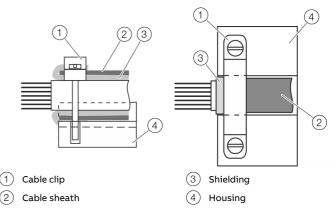
Figure 17: Cable shielding
