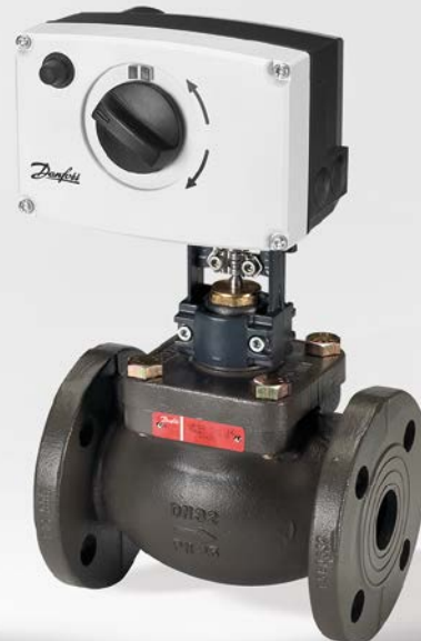
2-way seated valve VFS combined with AMV 25
