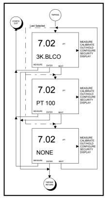
Figure 21 – Screen Flow Diagram for Temperature Sensor State of Operation
