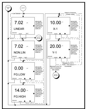
Figure 23 – Screen Flow Diagram for Linearity Type State of Operation
