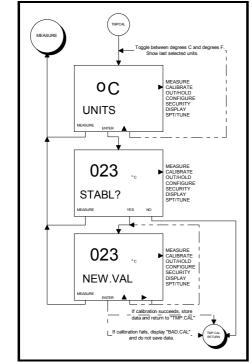
Figure 14 – Screen Flow Diagram for Temperature Calibrate State of Operation
