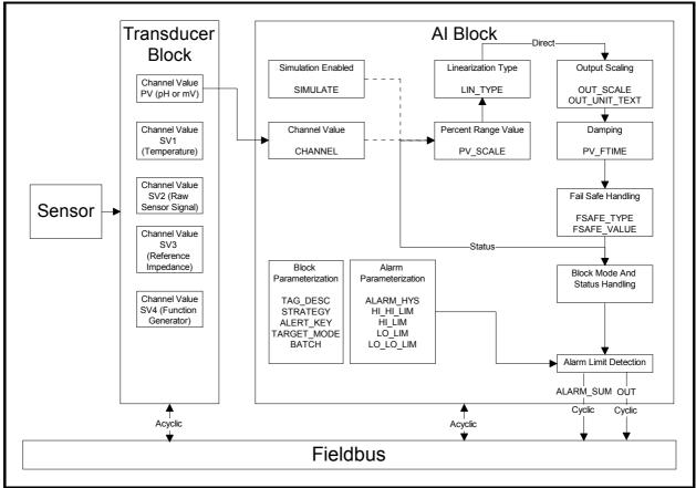
Figure 30 – Analog Input One Function Block Design Diagram
