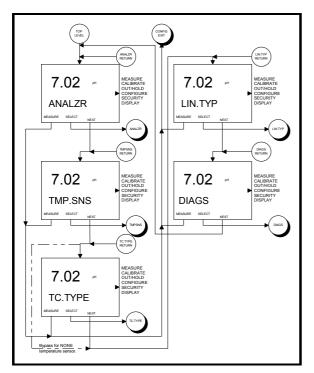
Figure 19 – Screen Flow Diagram for Modify Configure States of Operation
