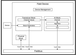
Figure 28 – Function Block Model Diagram
