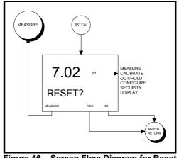
Figure 16 – Screen Flow Diagram for Reset Calibrate State of Operation
