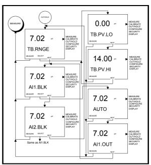
Figure 17 – Screen Flow Diagram for Output/Hold Mode and States of Operation
