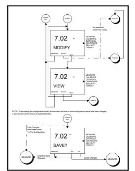
Figure 18 – Screen Flow Diagram for Modify/View and Save States of Operation
