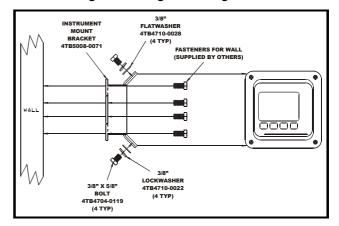
Figure 7 – Wall Mounting Detail
