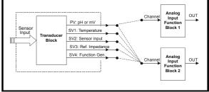
Figure 32 - Possible Connections Between the TB and Al's
