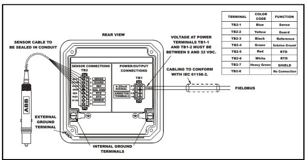
Figure 9 – Sensor and Power Wiring
