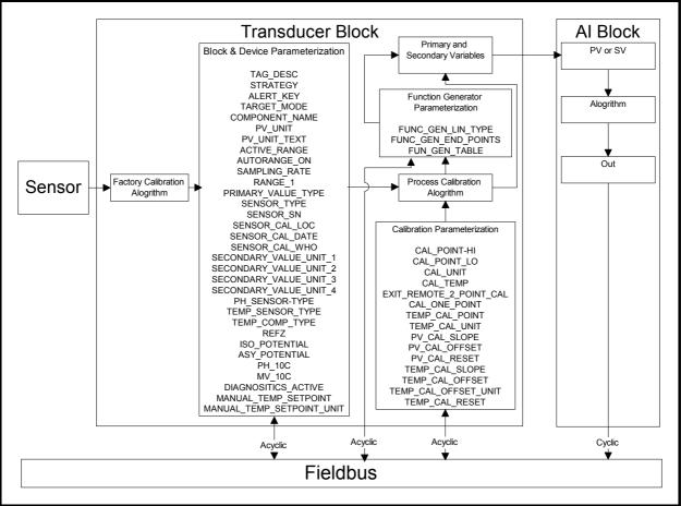
Figure 29 – Transducer Block Design Diagram
