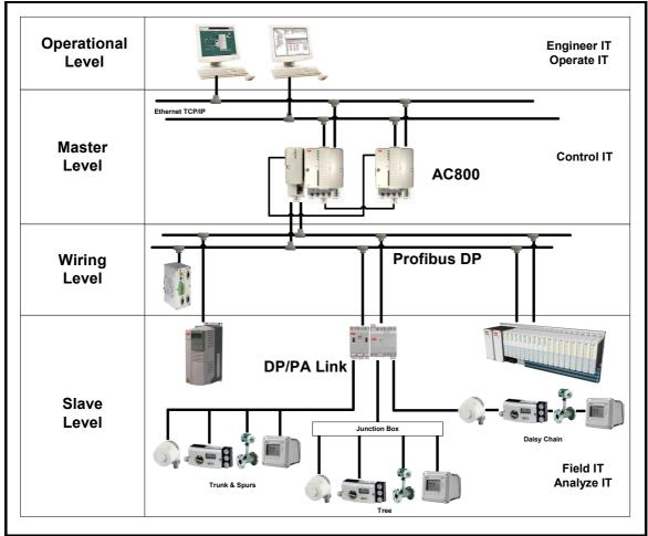
Figure 4 – Typical Bus Configurations
