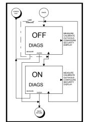
Figure 24 – Screen Flow Diagram for Diagnostic State of Operation
