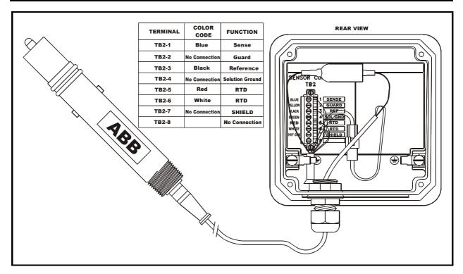
Figure 10 – BNC Adapter Sensor Connections
