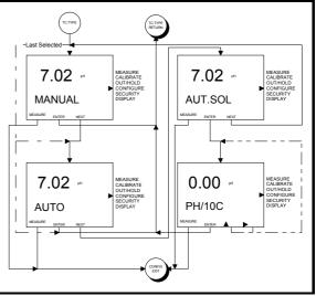
Figure 22 – Screen Flow Diagram for Temperature Compensation State of Operation.
