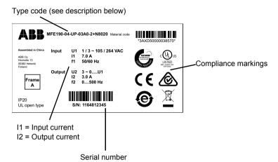
The first digit of the serial number refers to the manufacturing plant. The 2nd and 3rd digits indicate the year of manufacture, while the 4th and 5th digits indicate the week. Digits 6 to 10 are a running integer starting every week at 00001.
