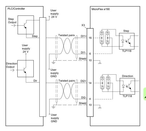
Step and direction inputs - typical connections from a PLC/controller using open collector outputs:
