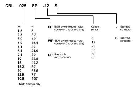
Larger motors requiring 35 A cable or greater normally use terminal box connections, so a motor power connector is not required. For this reason connectors are not available on 35 A - 90 A cable.
