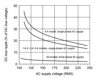
Effect of output current on DC-bus ripple voltage
