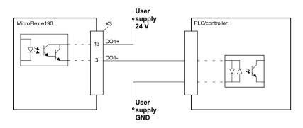
Digital output - typical connections to a PLC/controller:
