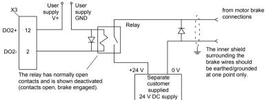
This circuit uses DO2 as a motor brake output. The output is configured using Mint keyword MOTORBRAKEOUTPUT; see the Mint help file for details. With this configuration, the following sequences can be used to control the brake.
