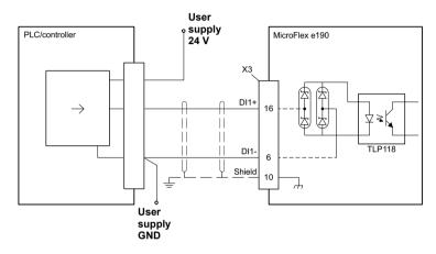
Digital input - typical connections from a PLC/controller:
