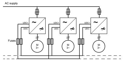
\* The MicroFlex e190 DC connection is not designed to provide the primary power source to other drives.
