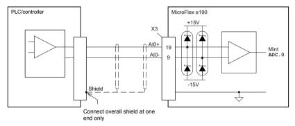
Analog input - typical connections from an ABB AO561:
