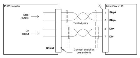
**Note:** The inputs should be use shielded twisted pair cable with an overall shield. Connect the input signals correctly according to the pin assignment for connector X7.
