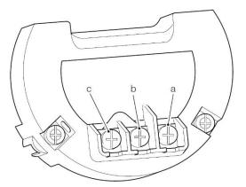
Figure 2. Terminals Introduction a Positive pole of power supply (+) b Negative pole of power supply (+) c Expansion table, short connection with negative pole in normal use (Ext)
