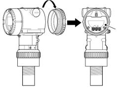
Figure 1. Cable Connection Area
