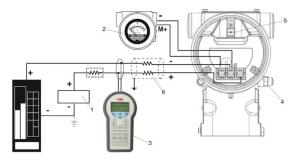
Fig. 3 Electrical Connection - HART Version 1. Power Supply
