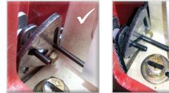
05 Remove the plastic bolts on the cover that supports the blown fuse switch.
