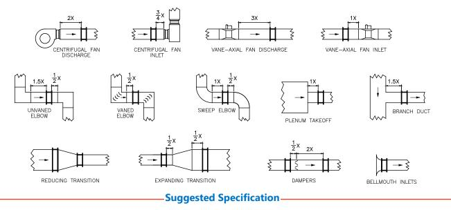
Provide at each indicated location a self-averaging Pitot traverse station with integral flow straightener-equalizer for continuous monitoring of the air volume flow rate in that line.
