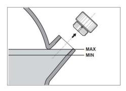
➤ Ensure the oil level in the Air End is between the top (maximum) or bottom (minimum) thread as shown.
