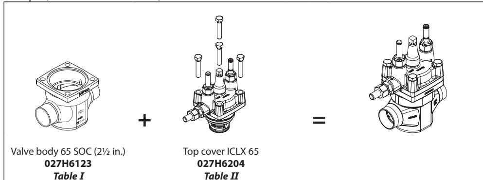
ICV 65 valve body w/different connections
