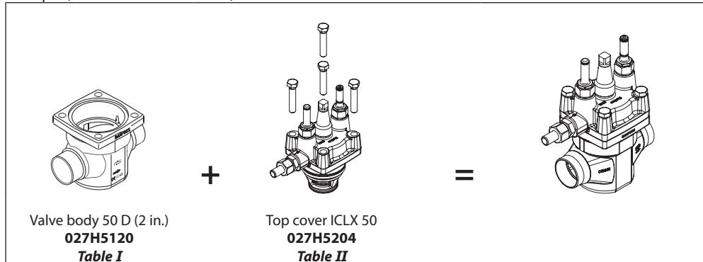
*ICV 50 valve body w/different connections*
