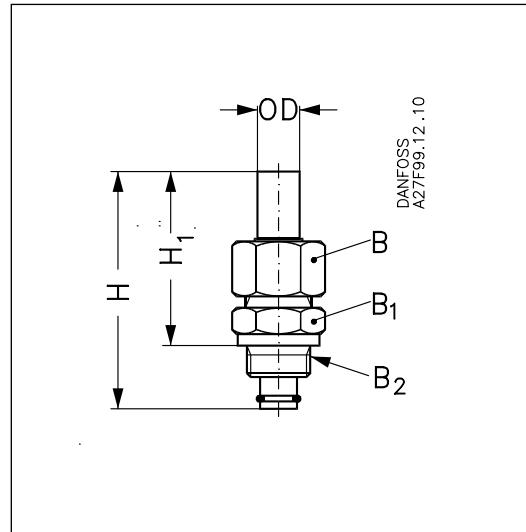
A damping orifice should be installed if the pressure difference between the low and the high pressure side is more than 6 bars.
