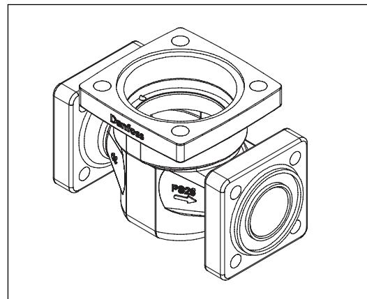
\*) Includes ICV PM valve housing, flange gaskets and flange bolts.
