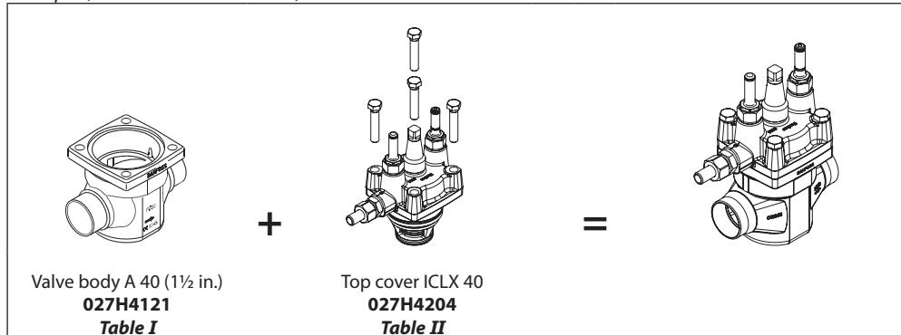
ICV 40 valve body w/different connections
