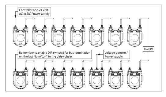
In case all BACnet devices are NovoCon® S, please see some examples for usage of voltage booster cable.
