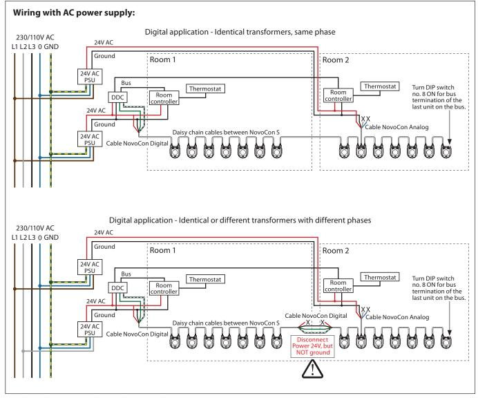
Wires that ends in an "X" must be properly terminated.
