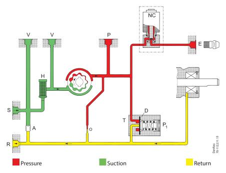
From the suction inlet (S) oil is drawn through the filter (H) to the gear set, where the pressure is increased. When voltage is applied to the NC-valve (normally closed), it opens and releases oil to the nozzle outlet.
