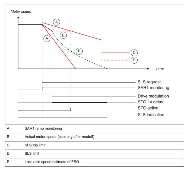
Example 3: SAR1 ramp monitoring and SLS modoff delay time active
