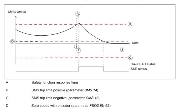
This time scheme diagram illustrates the operation of the SMS function (version 1).
