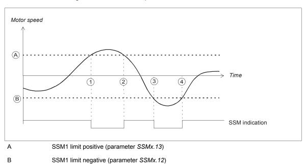
This time scheme diagram illustrates the operation of the SSM1 function.
