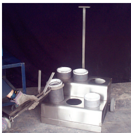
Reusable crucible trolley for safe cooling and easy saw carrying
