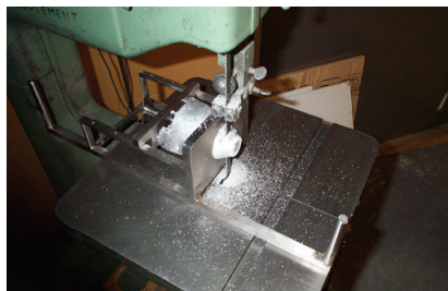
Metal sample holder for safe aluminum residue cutting on a band saw
