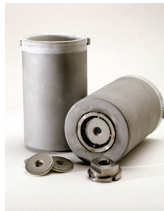
PoDFA reusable crucible and filter
