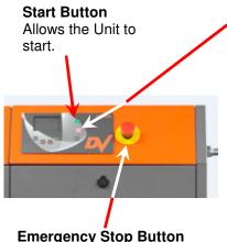
**Stop Button** Use this to shut the Unit off. Allows the Unit to idle and then stop after several seconds.
