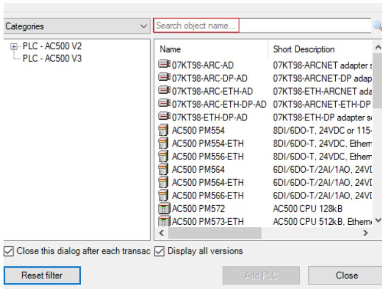
4. Check that the correct device type is selected by double clicking the device name in Devices field. Check that the correct Terminal Base Type is also selected for the tag for Hardware.
