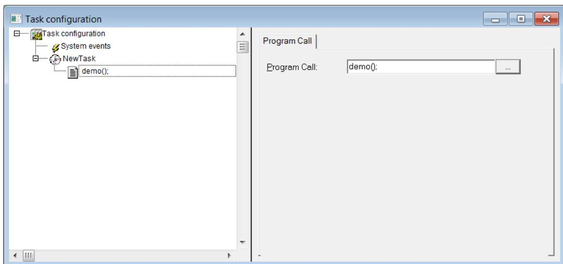
19. Now we can build the project by Project -> Build. Check again if fieldbus is connected correctly. We can then run the program by pressing ALT+F8 and then F5.
