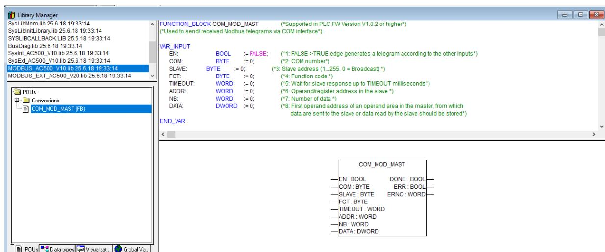
To enable this function block, it is required to send a FALSE->TRUE edge at input EN and therefore we introduce BLINK, which is for creating a flip-flop signal.
