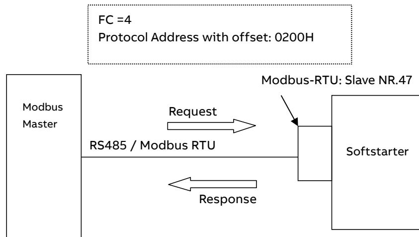
E.g: Read analog output words 2 & 3. Phase L1 current and Phase L2 current with default settings.
