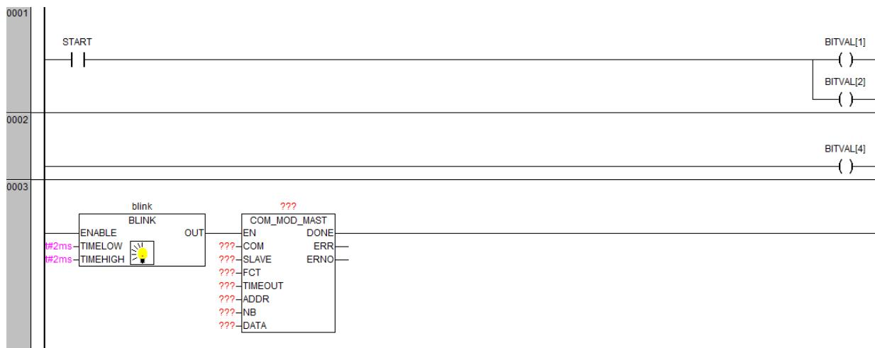
The COM\_MOD\_MAST is a function block for sending/receiving OpenModbus.
