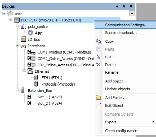
2. Control that the IP address for PC and the PLC is in the same network but not the same IP address. This can be checked by using through Ethernet Properties.
