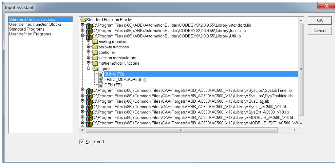
9. We name the BLINK function block as blink. We set t#2ms for TIMELOW and TIMEHIGH.
