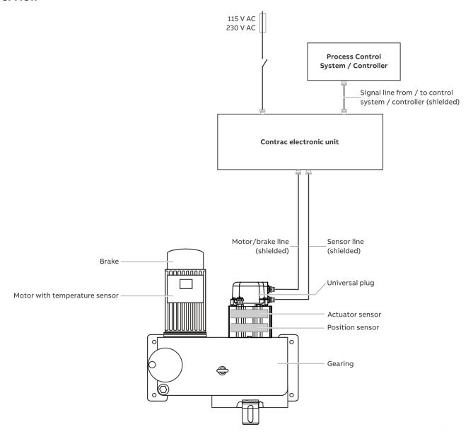
Figure 3: Structure of the Contrac components (example)
