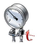
Close bypass and read pressure and process with flow indicator
